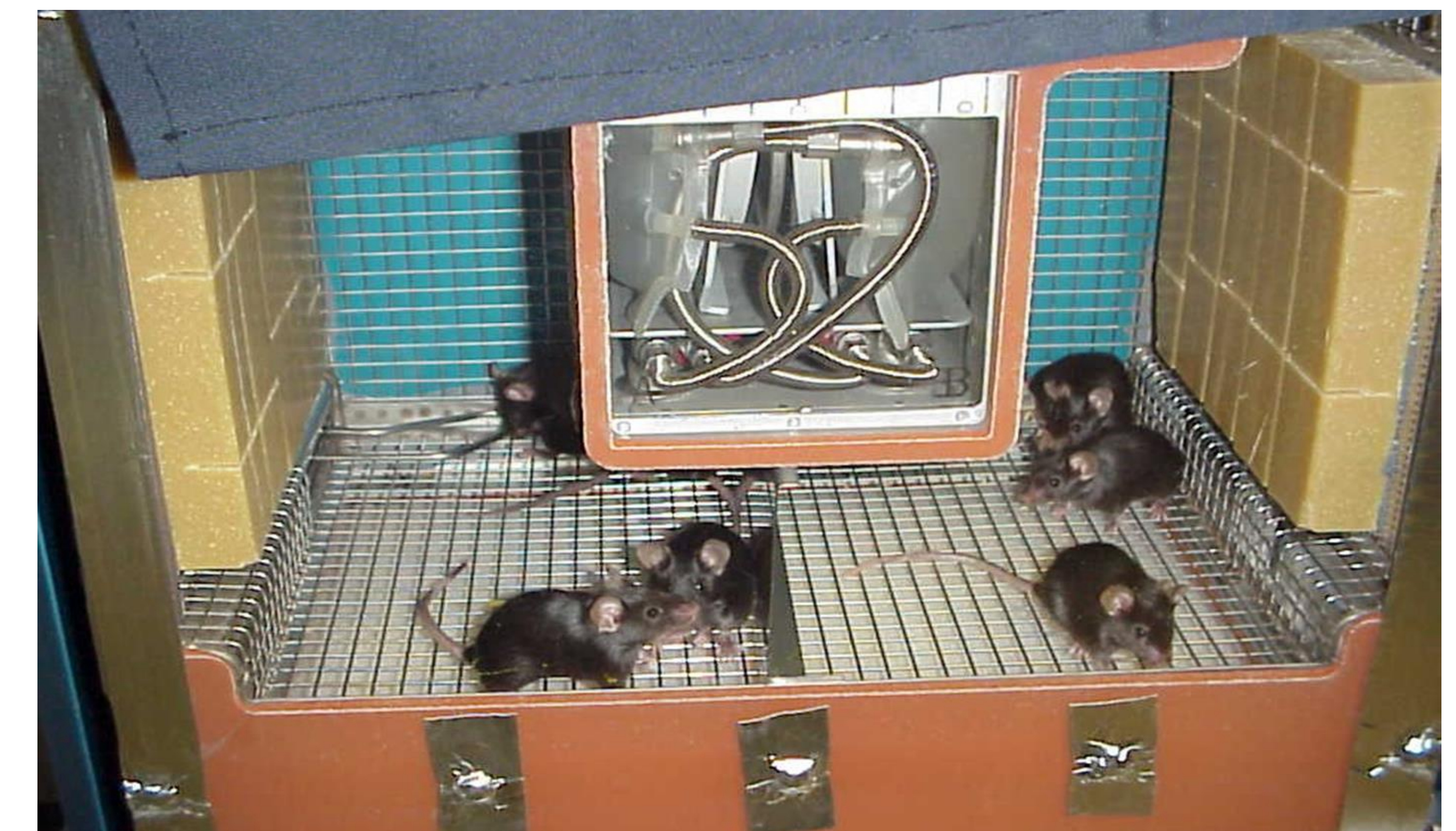
Figure 3. Flight habitat for mice. Shown are the habitats for mice in flight, with foodbars on the far walls and the water system in the center.
